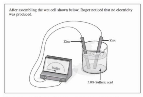
Which change could Roger make to the wet cell to produce electricity?
